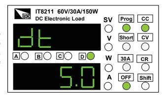
5) Press C View key to enter High Voltage setting, use cursor keys A ■ B ■ and the knob to set the high limit of the input voltage. Right figure set the HV as 60.00V.
