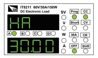
8) Press C View key to enter Low Current setting, use cursor keys <a> ■</a> and the knob to set the low limit of the input current. Right figure set the Low Current as 0.00A.
