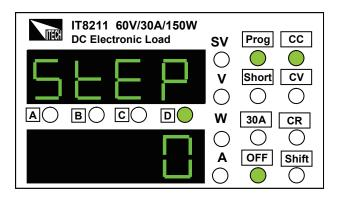
2) Press View key to enter TYPE setting. Use the knob to switch the working mode: CC mode, CV mode, CR mode. Right figure set TYPE as CC mode.
