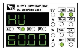
6) Press C View key to enter Low Voltage setting. use cursor keys and the knob to set the low limit of the input voltage. Right figure set the Low Voltage as 0.00V.
