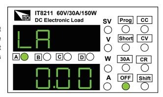
9) Repeat step 1 settings, in turn set 5 steps: 1/2/2V/5S/60V/0V/30A/0A;  $2/3/10\Omega/5S/60V/0V/30A/0A$ ; 3/1/2A/5S/60V/0V/30A/0A; 4/1/0A/5S/60V/0V/30A/0A (because the total steps is less than 25 steps, so the last step should be CC/0A.)
